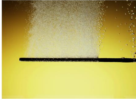
Figure 19: Pore Size Measured by Bubble Point Testing
